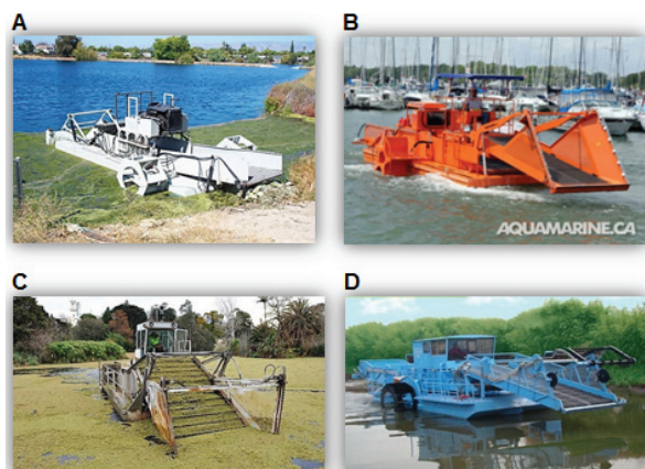
Fig. 1. The examples of manufactured harvesters for collection of aquatic vegetation and macroalgae (A–D) or cyanobacteria scums in small water bodies (E–F) and large water ecosystems (G–H). A – Harvester for aquatic vegetation and algae (San Jose, California, USA). https://commons.wikimedia.org/wiki/File:Algae_harvester-2.jpg [Accessed on 20-05-2019]; B – H5-200 Aquatic weed harvester Aquamarine H5-200 (Ontario, Canada). www.aquamarine.ca/aquatic-weed-harvesters/ [Accessed on 20-05-2019]; C – Azolla harvester (India). www.azollaamrit.com/gallery.php?pid=6 [Accessed on 20-05-2019]; D – SINOBE-ACON Automatic Underwater Aquatic Vegetation cutting device (China). 803768290/Specially_Designed_Automatic_Underwater_Aquatic_Vegetation_Harvester_For_Sale.html [Accessed on 20-05-2019]; E – ALGENT – mobile cyanobacteria harvesting platform (USA). www.smithsonianmag.com/innovation/startup-harvesting-wild-algae-make-your-next-pair-sneakers-180960872/ [Accessed on 20-05-2019]; F – ASIO – vessel for cyanobacteria harvesting (Czech Republic) www.asio.cz/en/vessel-for-the-separation-of-biomass-particles [Accessed on 20-05-2019]; G – Aphanizomenon flos-aquae scum harvester from Lake Klamath (USA). https://cerulequebecfr.com/tag/algue-klamath/ [Accessed on 20-05-2019]; H – modified oil boom device for harvesting cyanobacteria scums in the Baltic Sea, Sweden (GRÖNDAHL, 2009)
