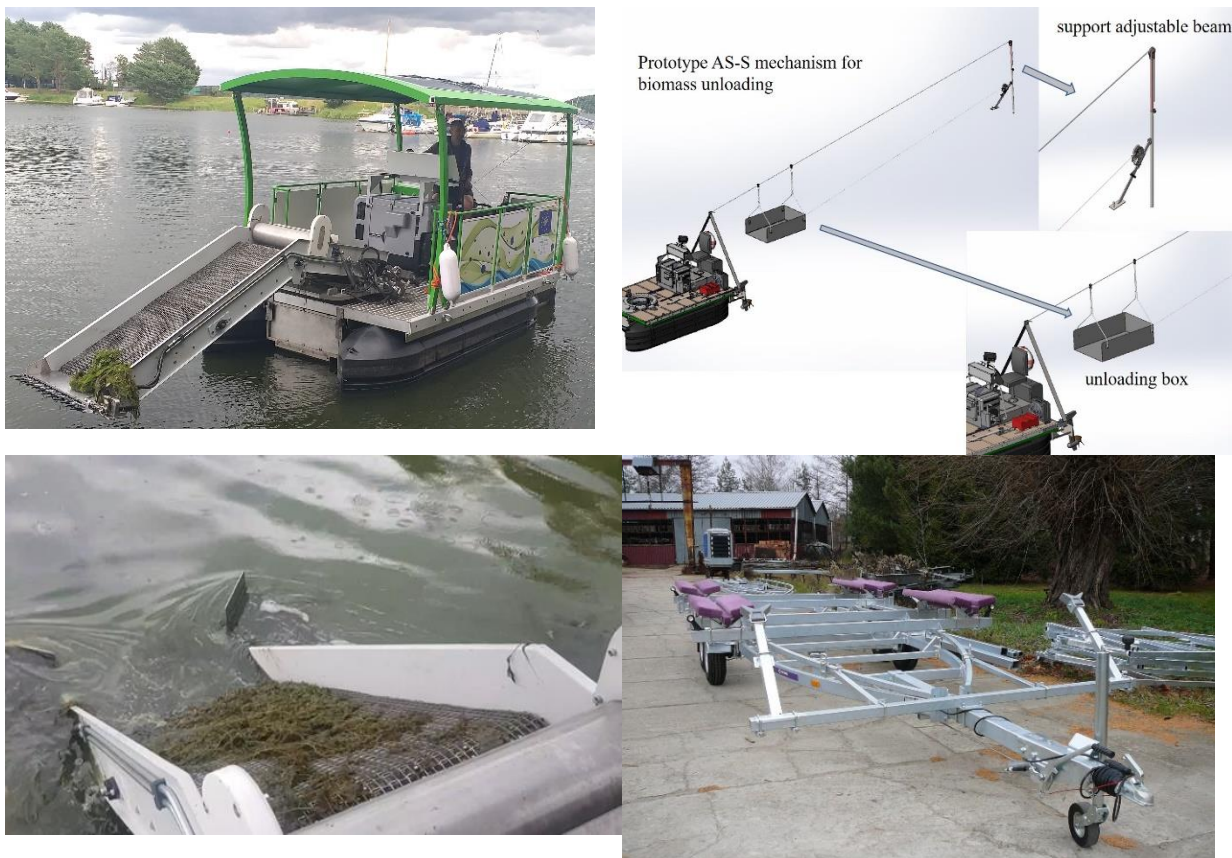
Fig. 4. Manufactured AS-S prototype, biomass unloading mechanism and custom-made trailer for prototype transportation
