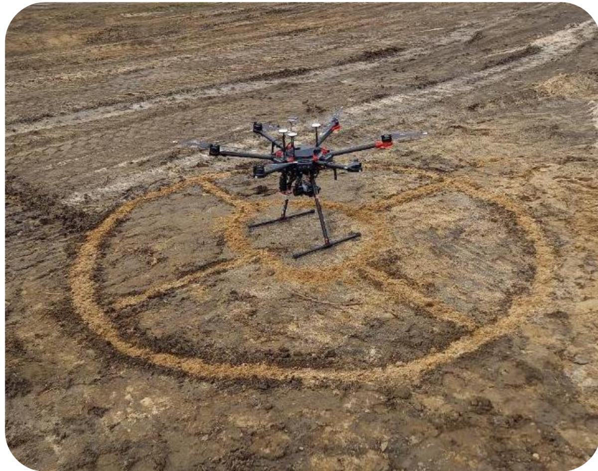
**2020 – MR UAV + 5 band multispectral camera + thermal camera**
