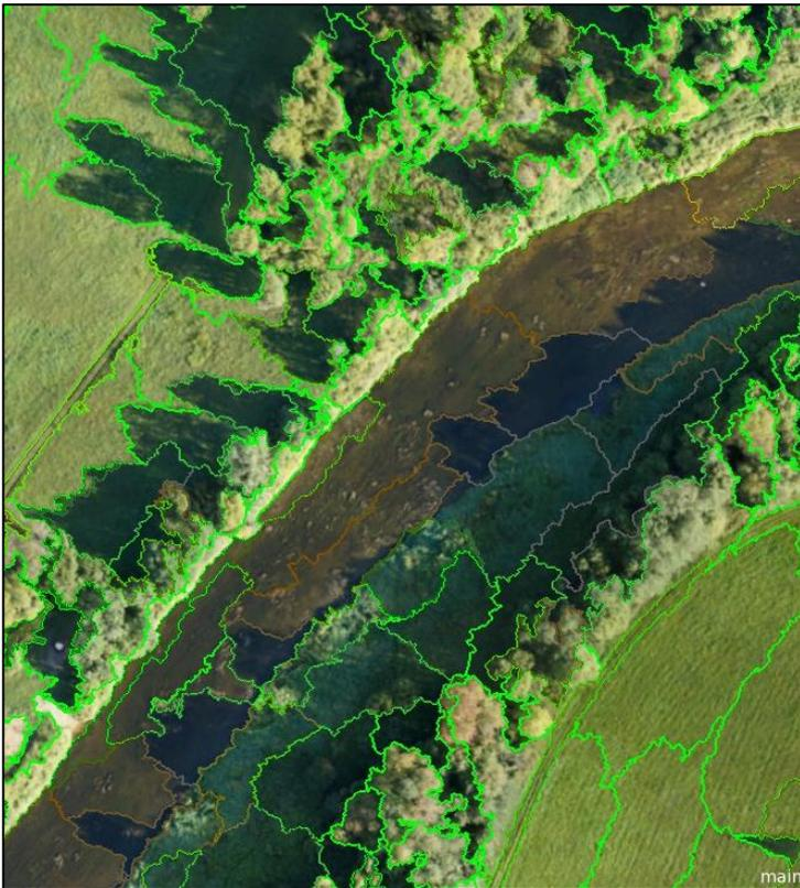
Segmentation and classification of riverbed according to bottom and surface properties:
