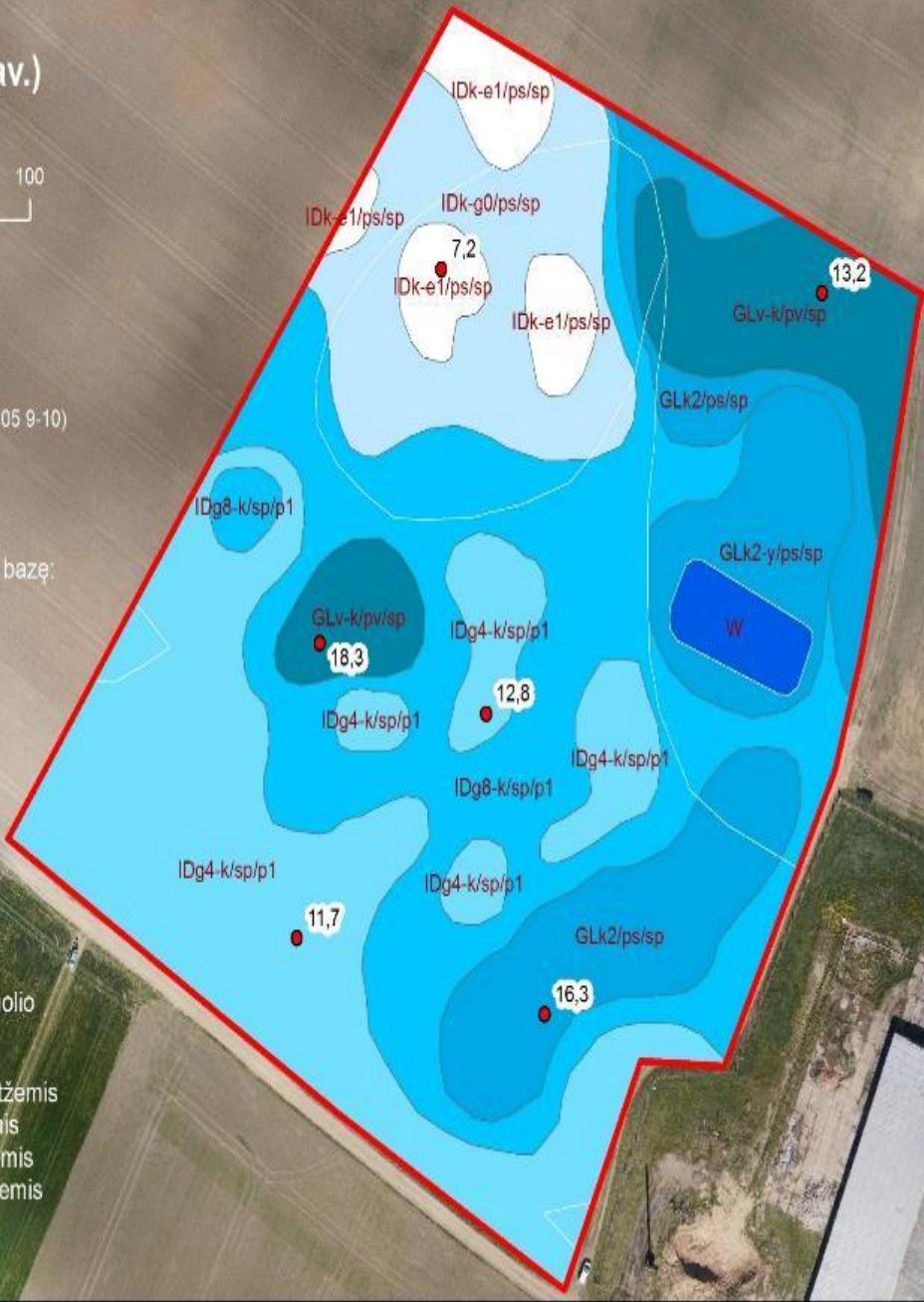
Soil typological mapping data are correlated with soil moisture data
