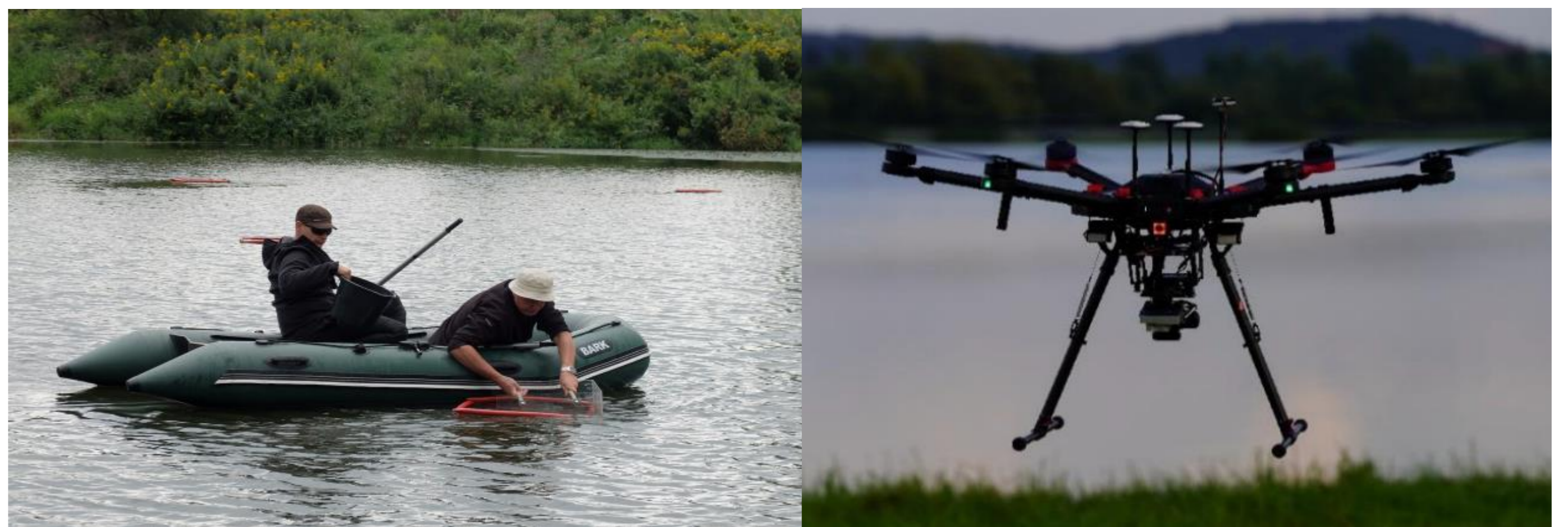
Fig. 1. Field works: deploying styrofoam frames on the surface of water (left) Fig 2. UAV used for remote multispectral analyses (right)
