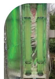
The installed photobioreactor for biogas upgrading:
