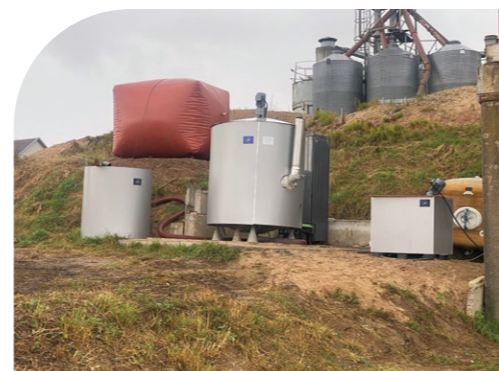
The installed photobioreactor for biogas upgrading:
