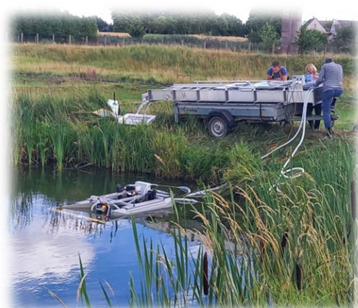
Fig. 3. Cyanobacteria biomass harvesting prototypes: AS-L (left) and AS-LAND (right)
