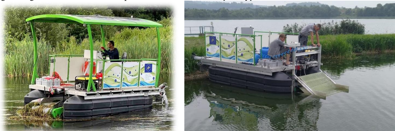
Fig. 2. AS-S prototype prepared for the collection of macroalgae mats (left) and cyanobacteria scums (right).
